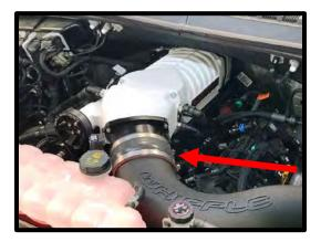
114. **(Stock throttle body installations)** Install the supplied reducer silicone hose over air inlet tube. Connect the other end to the stock throttle body. Secure all ends with the supplied hose clamps.
