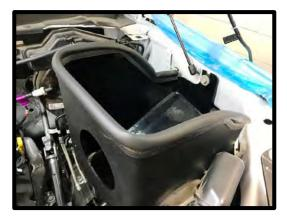
111. Install supplied rubber grommet into the Whipple air intake tube. Install the supplied aluminum barb to quick connect fitting into rubber grommet.
