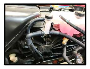
101. Connect the ¾" ID hose (#18F150-HS007) and the 3/8" ID hose (#18F150-HS008) hose coming from the IC filler neck to the ¾" and 3/8" barb fitting on the IC reservoir. Secure with supplied pinch clamp. **NOTE: Ensure that this hose cannot kink or rub anything overtime.**
