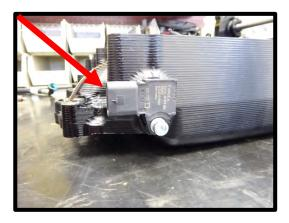
51. Pre-install the supplied MAP pigtail to the new MAP sensor.
