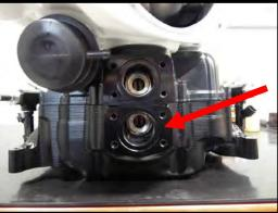
72. Install the supplied #126 oring to the manifold bottom intercooler passage location. Apply light amount of grease to oring to help secure in place. Install the supplied intercooler hose connect fitting to lower intercooler passage. Apply light amount of blue Loctite #243 to threads of the supplied (2 of 4) 6mm x 10mm FHSCS.
