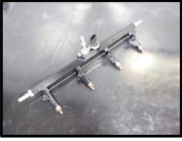
48. Mount fuel rails to intake manifold using the (4) 32mm long spacers between the manifold and fuel rail boss and the (4) 6mm x 50mm SHCS, apply light amount of blue Loctite #243 to threads. Torque to 90 in-lbs using a 5mm allen socket.
