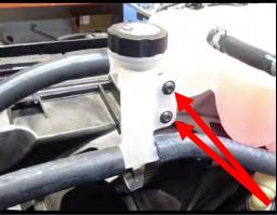
104. Install the ¾" ID rubber hose (#18F150-HS006) from the top IC fitting (outlet) to the IC filler neck. Secure both ends with supplied pinch clamps.
