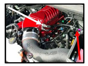
106. Install the supplied throttle body oring to the supercharger inlet. Apply light amount of grease to help hold in place.
