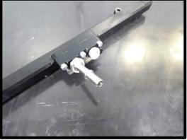
46. Install the supplied -6 orings to the (4) inlet/outlet fittings. Install these (4) fittings into each side of the fuel rails. Apply light amount of grease to oring for ease of installation. Using a ¾" wrench (or ¾" deep socket) on both the front and rear fittings, tighten both.
