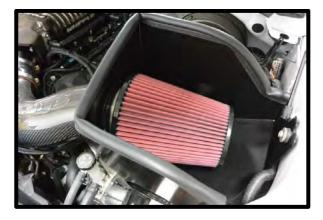
113. (Whipple 132mm Crusher throttle body) Install the supplied 5" ID x 2" silicone hose over air inlet tube so it's not hanging over the end. Install the air inlet tube between the filter and throttle body. Slide silicone hose over throttle body. Secure all ends with the supplied #80 hose clamps.
