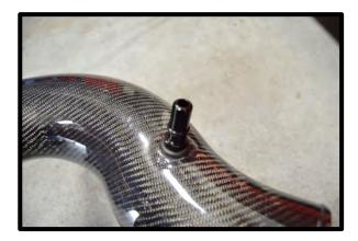
112. Slide the Whipple air intake tube through the airbox, install the supplied high flow filter to tube and secure hose clamp using a 5/16" nut driver.
