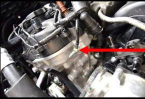
38. Cut the ground wire you previously removed from passenger side of cylinder head stud. Route wire along factory harness (will zip tie later) up towards the valve cover. Slip the supplied heat shrink over the ground wire. Strip the end of the supplied ground wire and the engine ground wire. Install the supplied butt connector, crimp both ends. Slide the heat shrink over the butt connector and apply heat to seal.
