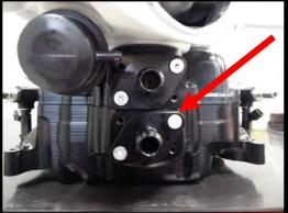
73. Install the supplied ¼" ID bypass actuator hose (#18F150-HS005) to the bypass nipple and ¼" nipple above first cylinder on driver side.
