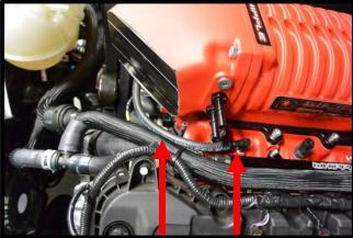
74. Using a razor blade, carefully cut the 90deg and 45 deg quick connect fittings from the factory PCV line. Install these fittings into the supplied 1/2" x 7" hose (#18F150-HS004). Install the ¾" x 8" sleeving and heat shrink to the ½" x 7" hose. Shrink sleeving and heat shrink, using the heat shrink material to cover the cut ends of the hose.
