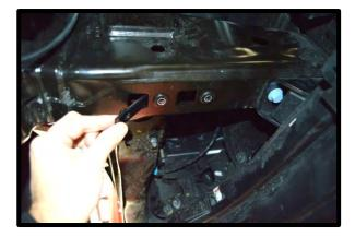
97. Install the IC reservoir to the (2) nut plates using the (4) 8mm x 25mm flanged hex headed bolt. Start (1) on each side to align holes to bushing. If off, you can use screwdriver to align the nut plate and bushing before installing the final (2) bolts. Torque to 15 lb-ft using a 13mm socket.
