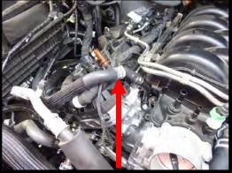
22. Install the supplied driver side heater tube to passenger side of block. Install the supplied oring to the tube and apply light amount of grease to oring surface. Install tube into block and secure with the factory bolt using an 8mm socket. Torque to 89 lbs-in.
