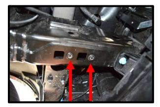
96. Install the supplied steel nut plates (2), (1) per side up through square opening with nuts facing up.
