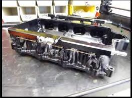
49. Install the rear pre-made cross-over fuel line. Press until the click and lock into position.
