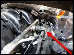
25. Using a 3/8" fuel line removal tool, remove the feed line from the factory port injection system to the direct injection mechanical pump. Slide removal tool between the lines, securing the DI side until it releases. NOTE: THIS FUEL LINE HAS A CHECK VALVE, DO NOT FLIP ORIENTATION. DO NOT REMOVE FROM DI PUMP TO ELIMINATE CONFUSION. 90-DEG END ALWAYS CONNECTS TO FUEL FEED SUPPLY!
