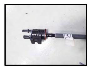
70. Install the supplied -6 orings (4) to the inlet fittings. Apply light amount of grease to the orings for ease of installation. Install the 15.82 to 6 ORB to the passenger side inlet open thread. Install the (2) 9.89 to 6 ORB fittings to the driver side inlet open threads. Install the 6 ORB plug in the middle thread.
