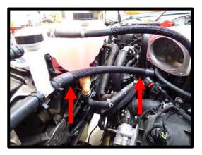
105. Install the supplied 15/32" (#F150-2000) brake booster hose to the factory check valve. Route this line up to the front of the driver side valve cover (secure with 2 zip-ties to factory wire harness). Connect 90deg quick connect to bottom fitting in the supercharger inlet. Push until it clicks into place.
