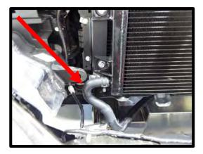
99. Connect the ¾" ID molded/formed (33") hose (#18F150-HS009A) from the LTR driver side bottom fitting that you previously installed, to the IC pump outlet barb. Secure with supplied pinch clamp. **NOTE: Ensure that this hose cannot kink or rub anything overtime.**
