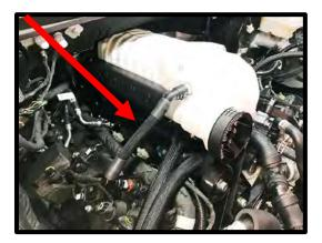
76. Install the supplied 3/8" x 8 ½" EVAP hose (#18F150-HS002) to the EVAP solenoid and bottom inlet fitting.
