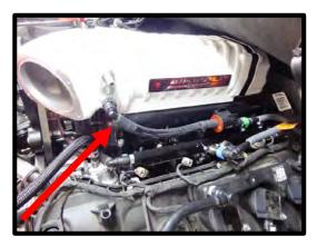
77. Install the supplied electronic throttle pigtail to the factory electrical connector. Push until it locks in place, then lock the safety lock. Leave near the thermostat housing for later connection to throttle body.
