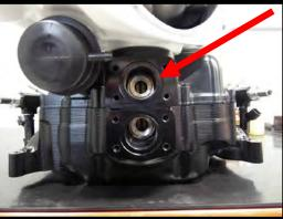
67. Install the supplied #126 Viton oring to the manifold top intercooler passage location. Apply light amount of grease to oring to help secure in place. Install the supplied intercooler hose connect fitting to upper intercooler passage. Apply light amount of Blue Locite #243 to threads of the supplied (2 of 4) 6mm x 10mm FHSCS.
