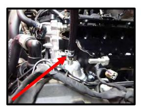
61. Install the supplied front fuel cross over line to the front until they click and lock in place. The 90deg end goes on driver side fitting. *Route behind water neck vent line*. *Ensure that its free from rubbing anything during engine vibration*.
