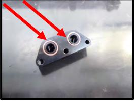
43. Using a 27mm socket, remove the fuel PSI sensor from the factory fuel rail. Install the factory fuel PSI sensor to the adapter using a 27mm socket. Torque to 53 lbs-in, then an additional 25 degree rotation. \*No sealant on the threads.
