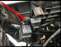
117. Using a 10mm socket, remove the nut on the power stud, located on the positive battery connector. Install the IC pump relay power eyelet (red wire) to the power stud on the battery positive (+) stud. Use a 10mm socket to secure stock and IC power wire.
