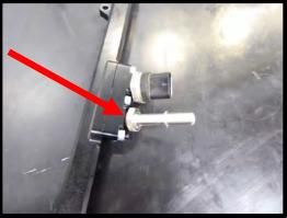
45. Install the supplied (1) -6 oring to the (1 of 2) 45mm long 9.49mm outlet fitting. Apply light amount of grease to oring for ease of installation. Install fitting to the fuel inlet block. Install the supplied -6 ORB plug to the extra port.
