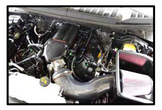
115. Secure the supplied (COYO-2000) driver side valve cover vent line quick connect fitting to the 5/8" fitting in the inlet tube previously installed.
