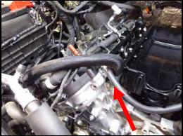
63. Cover the (1) IMRC solenoid and (2) IMRC position sensor connectors with electric tape and secure to the factory loom at the back of the engine.
