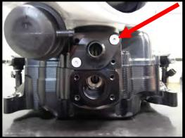
68. Carefully install the supercharger assembly to the intake manifold. Install the EVAP bracket to the 3 and 4 bolts (driver side from front) bolt bosses. Use the supplied (10) 8mm x 30mm SHCS and (2) 8mm x 60mm SHCS to secure SC assembly (6mm allen socket). Torque the supercharger bolts in an inside-out, crisscross pattern. Torque all bolts to 13 lbs-ft. on first pass, 17 lbs-ft on second pass.
